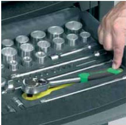
»Push-out« recesses ease removal of tools and speed up work.
